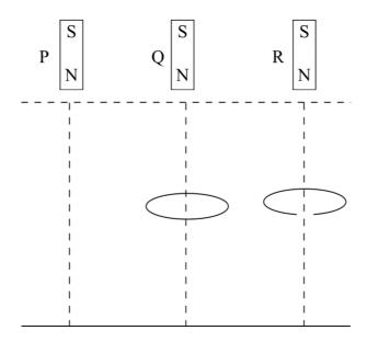
Three identical magnets P, Q and R are released simultaneously from rest and fall to the ground from the same height. P falls directly to the ground, Q falls through the centre of a thick conducting ring and R falls through a ring which is identical except for a gap cut into it. Which one of the statements below correctly describes the sequence in which the magnets reach the ground?
