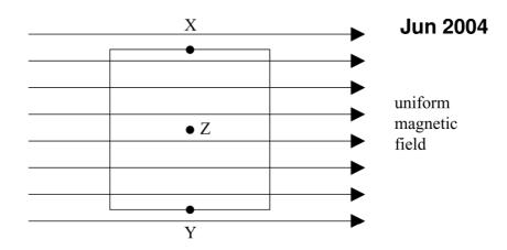
The diagram shows a square coil with its plane parallel to a uniform magnetic field. Which one of the following would induce an emf in the coil?
