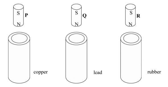
Three vertical tubes, made from copper, lead and rubber respectively, have identical dimensions. Identical, strong, cylindrical magnets P, Q and R are released simultaneously from the same distance above each tube. Because of electromagnetic effects, the magnets emerge from the bottom of the tubes at different times.
