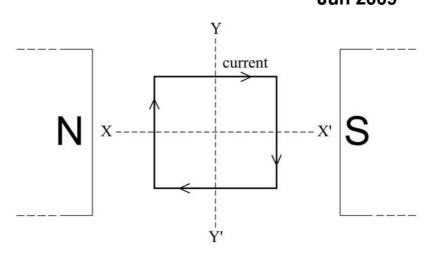
When a current is passed round the coil in a clockwise direction,
