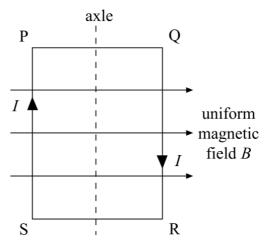
A coil, mounted on an axle, has its plane parallel to the flux lines of a uniform magnetic field B, as shown. When a current I is switched on, and before the coil is allowed to move,
